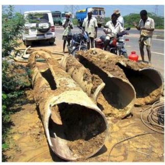
The pipelines were damaged by mechanised road cutters —Photo: Special Arrangement Telecom major Reliance Infocomm, which was responsible for the damage of pipelines transporting water from the dry bed of Palar river while laying telephone cables last month, is yet to pay a fine for the damage. This was revealed in a reply to a query under Right to Information Act.
